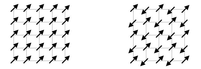
Figure 2: Average spin directions in phases with (a) ferromagnetic and (b) antiferromagnetic order on the square lattice. (The ordering direction is arbitrary.)
