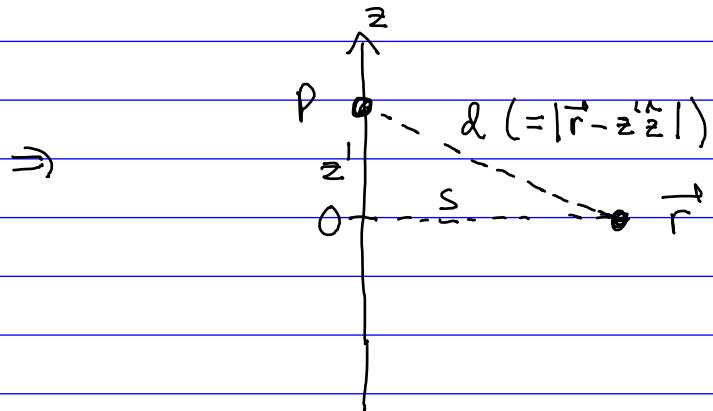
A point  $P$  on the wire at  $\vec{r}' = z'\hat{z}$  is at distance  $d = \sqrt{z'^2 + s^2}$  from  $\vec{r}$ . For  $P$  to contribute to  $\vec{A}$  at  $(\vec{r}, t)$  requires  $d \leq ct$
