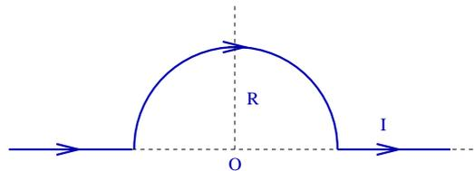
An infinitely long wire carries a (time-independent) current  $I$ . The wire is bent so as to have a semi-circular detour, of radius  $R$ , around the origin  $O$  (see figure).
